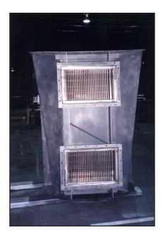
the Thermo-Z, they capture heat from the flue gases coming out of the liquid heater's exhaust at 680°F and use it to preheat combustion air going into the heater at 365°F. The heat exchanger increases the efficiency of the heater by 10%, saving the customer an equivalent amount in fuel.
