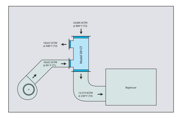
At a large midwestern printing plant, solvents used in ink from presses generate harmful vapors. Two regenerative thermal oxidizers, with a combined 70,000 CFM exhaust, incinerate the VOCs. But rather than let all that heat go to waste up a stack, the company wisely uses it to heat its facility.
